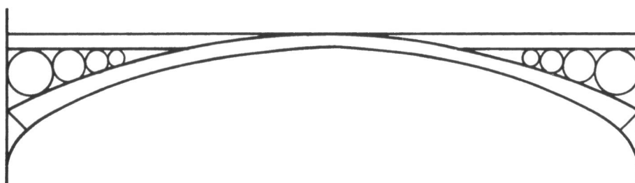
Fig. 6.4 Schematic diagram of wrought-iron bridge.
